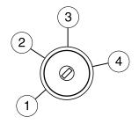
engine begins cranking. Your vehicle has a computer assisted cranking system that assists in starting the engine. After releasing the key from the 4 (start) position, the engine may continue cranking for up to 10 seconds or until the vehicle starts.
